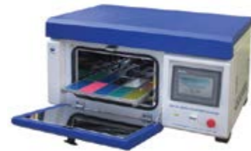
Small Xenon Test Chamber with spray function
