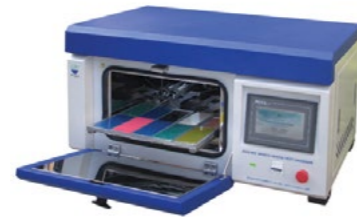
Small Xenon Test Chamber with spray function
