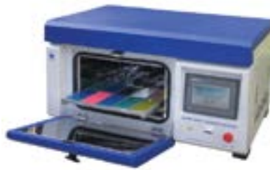
Small Xenon Test Chamber with spray function
